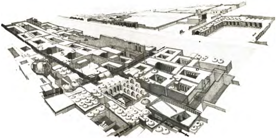
Fig. 2 – Yazd. This detailed drawing of the portion numbered 3 in the air photo of Yazd / Fig. 1 shows how the 30 meter-wide avenue cut away a large strip of the town fabric.
